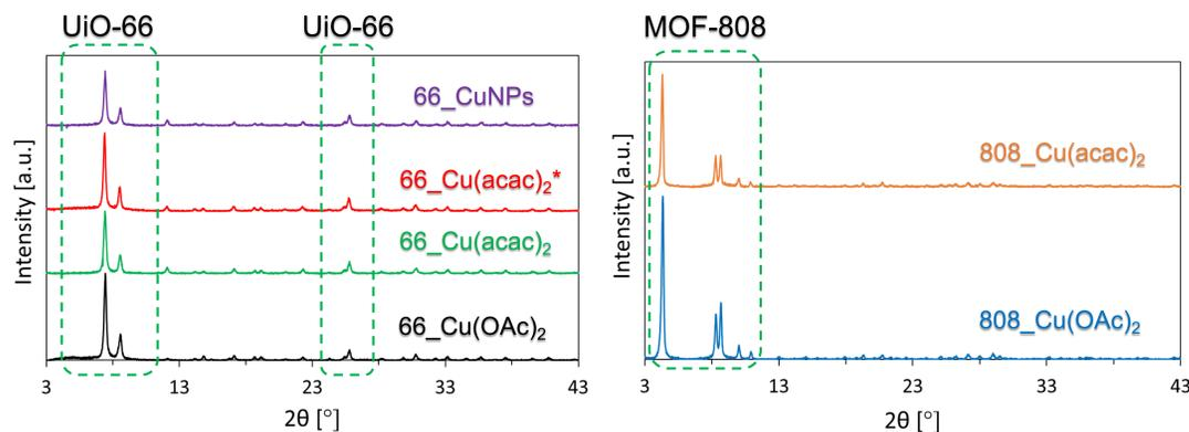
✓ Composites maintained crystalline structure after the Cu introduction process. ✓ No additional, undesired phases were observed.
